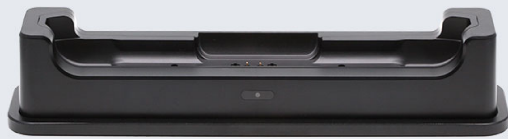
CRD-P80-RBC Charging Cradle for device, use with DCPWR-12V2A-XX adapter. The cradle cup has an insert that is fixed by 4 pcs screws and they must be removed in prior when charging P80 with rugged boot.
