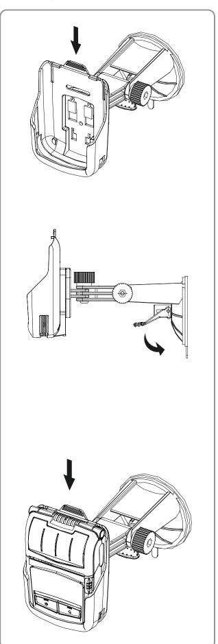
1) Assemble the vehicle holding cradle to the mount.
