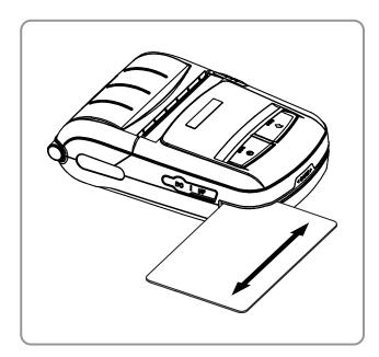
Insert the card as shown in the image and swipe in the direction of the arrow. (can be done in both directions)
